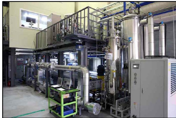
Figure 1. Flow Accelerated Corrosion Testing System (FACTS).
