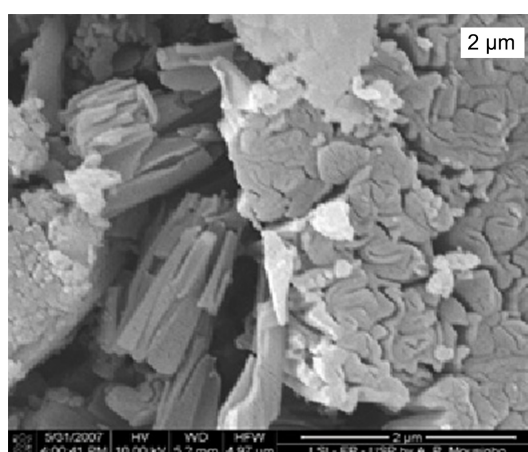
Figure 8. SEM micrograph of fractured surface of SWCNTs after 3 hours deposition time.
