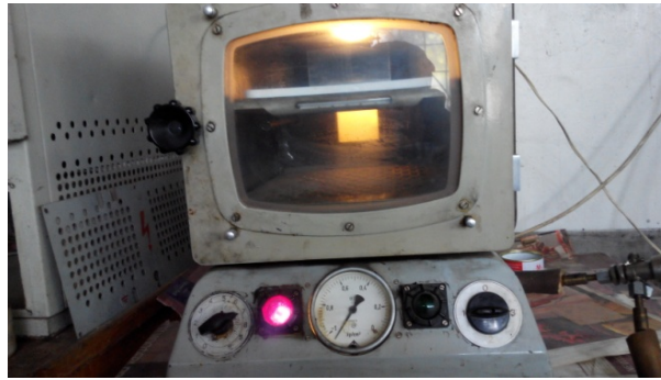
Figure 3. The vacuum cabinet with samples under the testing.
