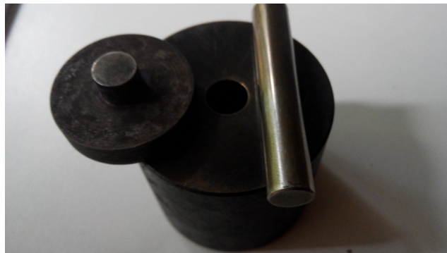
Figure 6. Press form for samples fabrication.
