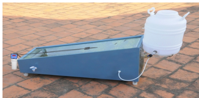
Figure 2. Solar still made up of copper.
