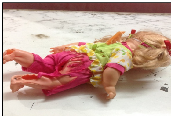
Figure 6. Plastic of the toy melt but did not burn.
