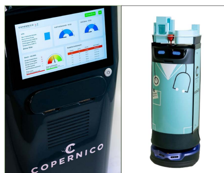
Figure 1. “COPERNICO Surveillance & Prevention” robotic system with integrated display to monitor the hygiene robotic intervention and collect data.
