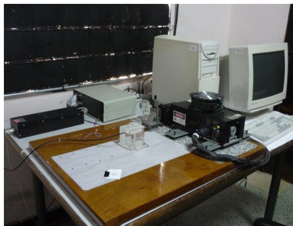
Figure 4. Meridialysis CZE ® system (model 3ZPO). It is equipped with an argon laser to induce fluorescence from samples that run through capillary electrophoresis.
