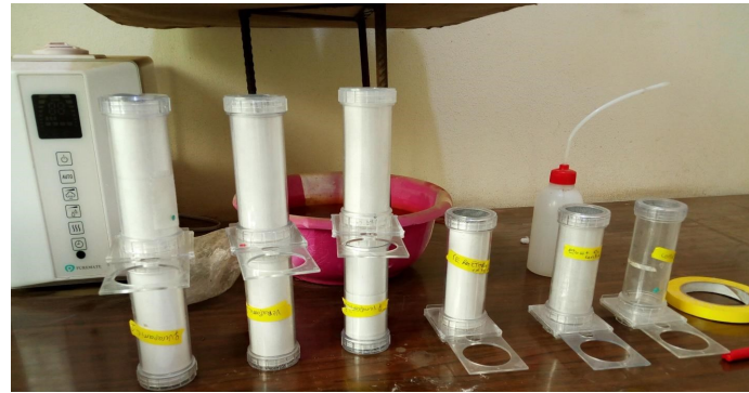
Figure 2. WHO bioassay. 1, 2 & 3: pre-exposure to verapamil treated papers and then 0.75% permethrin; 4: Permethrin treated papers alone; 5: a control paper with ethanol + Dow Corning oil; 6: 6 control of untreated paper).
