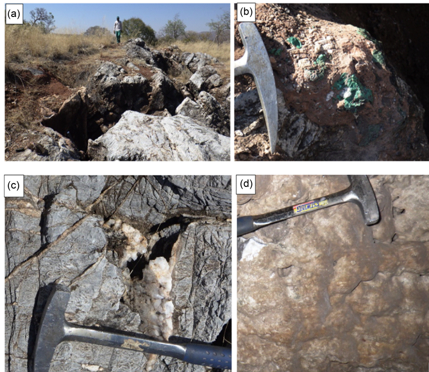
Figure 9. OMEG Gross Otavi pits observations; (a) historically mined narrow pits (looking towards the west direction); (b) matrix-supported breccia deposit of chalcocite, malachite and hematite ore; (c) euhedral to subhedral quartz crystals within the quartz veins; (d) botryoidal-shaped unit of brownish calc-silicate in the Gross Otavi adit.
