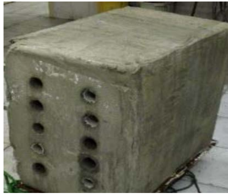
Figure 2. Concrete block including 10 holes.
