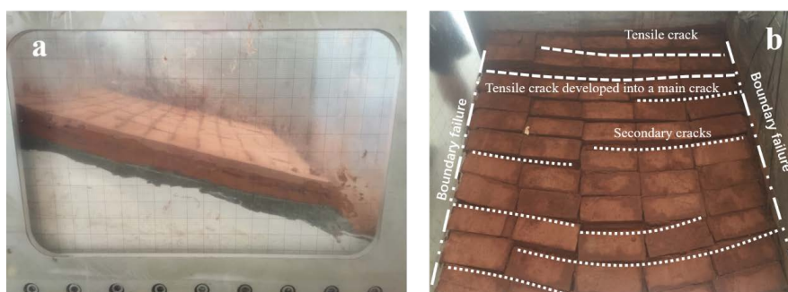
Figure 5. (a) The model before the centrifuge test; (b) The model after the rainfall condition centrifuge test, showing the overall slope instability that emerged.
