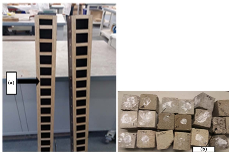
Figure 4. (a) Parametric casting boxes; (b) Some tested sample blocks.
