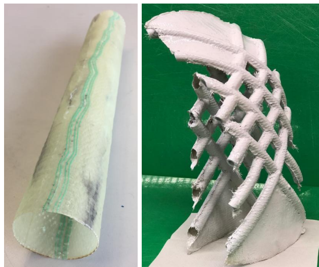
Figure 14. Pictures of hollow cylinder and hollow network flat and curved composite assembly.
