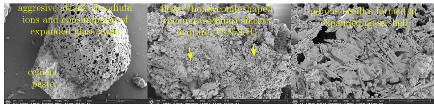
Figure 13. SEM images of 26-hour mortar with expanded glass as aggregate and 20M NaOH aqueous solution mixed with cement as the binder (sample U1 in Table 3 ) exposed to ultra-accelerated ASR regime.
