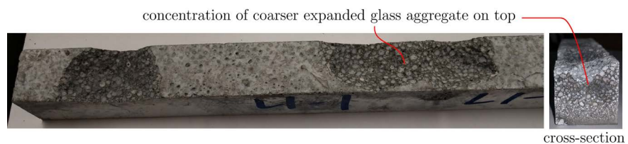
Figure 9. Spalling of the mortar bar in the sample with expanded glass where coarser aggregates are present. Sample was exposed to 1M NaOH solution for 68 days.
