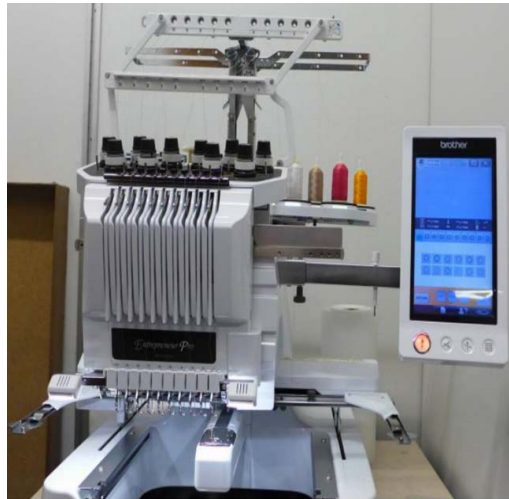
Figure 2. Brother Pr1000e embroidery machine at Loughborough university.
