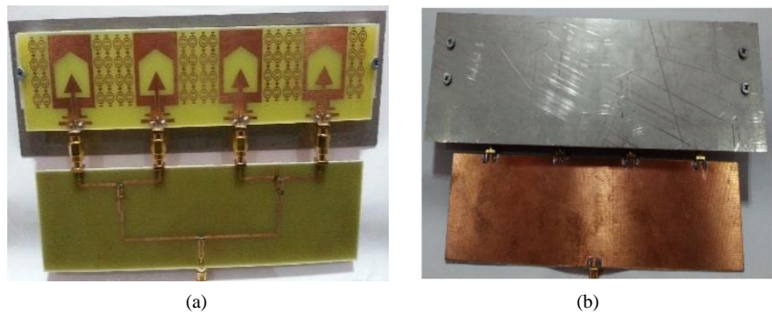
Figure 11. The fabricated antenna array (a) front side and (b) back side.
