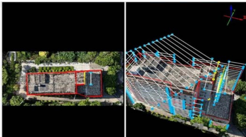
Figure 2. Schematic diagram of the route planning for the drone close-up photography.
