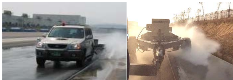
Figure 9. Hydroplaning test in proving ground.
