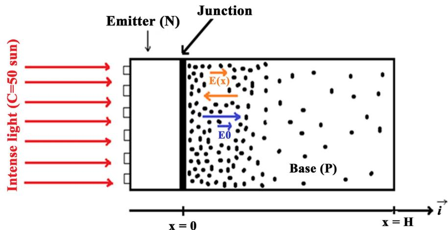
Figure 1. PV cell under concentrated illumination and under external electric field.
