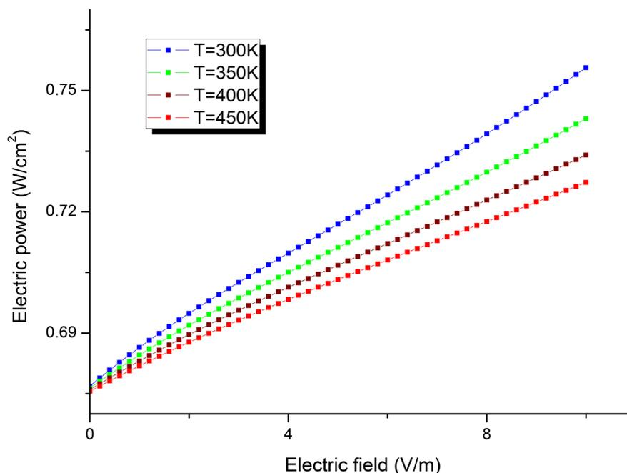
**Figure 4.** Variations of the electrical Power versus electric field and the temperature of the base ( $S_r = 5 \times 10^5$  cm/s;  $S_b = 10^3$  cm/s;  $H = 0.03$  cm;  $C = 50$  suns).
