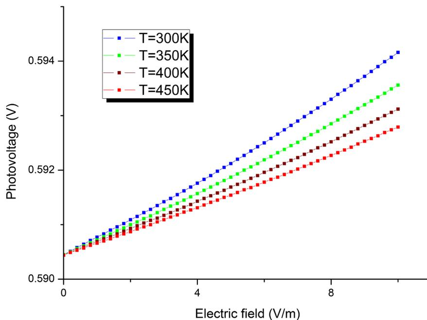
**Figure 3.** Evolution of the photovoltage versus electric field and the temperature of the base ( $S_f = 5 \times 10^5$  cm/s;  $S_b = 10^3$  cm/s;  $H = 0.03$  cm;  $C = 50$  suns).
