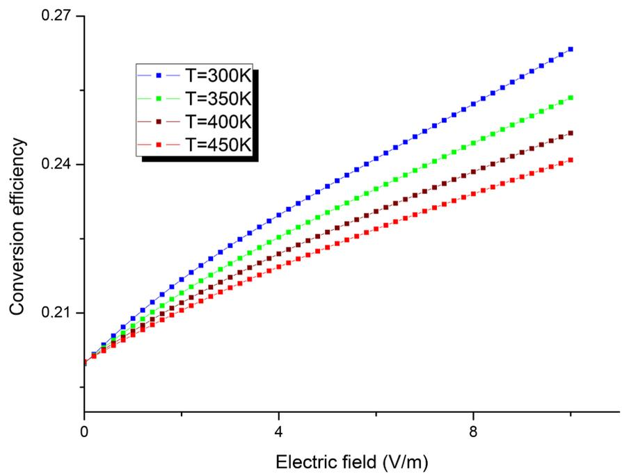
**Figure 6.** Variations of the conversion efficiency versus electric field and the temperature of the base ( $S_r = 5 \times 10^5$  cm/s;  $S_b = 10^3$  cm/s;  $H = 0.03$  cm;  $C = 50$  suns).
