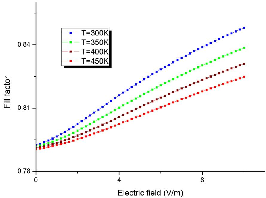
**Figure 5.** Variations of Fill Factor versus electric field and the temperature of the base ( $S_r = 5 \times 10^5$  cm/s;  $S_b = 10^3$  cm/s;  $H = 0.03$  cm;  $C = 50$  suns).
