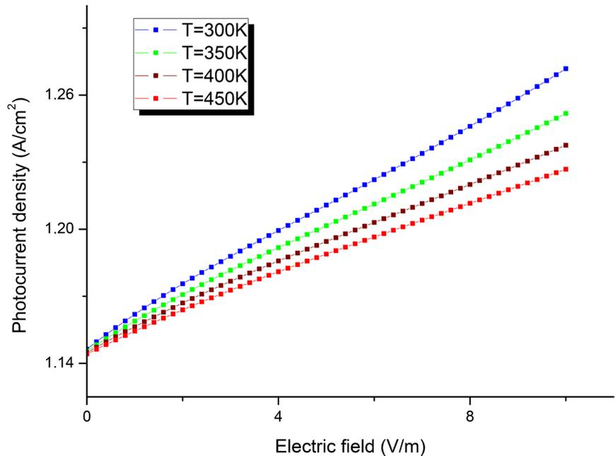
**Figure 2.** Variations of photocurrent versus electric field and the temperature of the base ( $S_F = 5 \times 10^5$  cm/s;  $S_B = 10^3$  cm/s;  $H = 0.03$  cm;  $C = 50$  suns).
