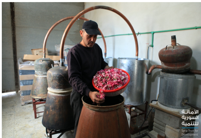
Figure 7. The distillation of the roses through copper distilleries called Alkirkh placed over a fire after adding water to the petals and waiting for the boil. Rose water is then placed in vials until it is ready for use. © Courtesy of the Syria trust for Development, 2016.
