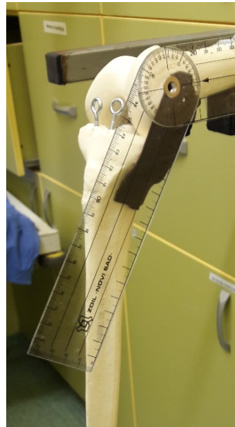
Figure 2. Sawbones® models with different extra articular starting points and measuring the bending angle in one model.
