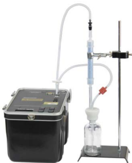
Figure 1. A typical setup of the DurrIDGE RAD7 radon detector with the attached RAD H 2 O accessory showing a 250 ml sampling bottle and tube of the DRIRITE desiccant.
