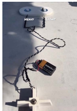
Figure 3. This apparatus has a manual switch that controls what side and for how long the shock is administered. The switch and base are connected by wires to one platform consisting of two separate wells filled with 50% sucrose by volume solution.
