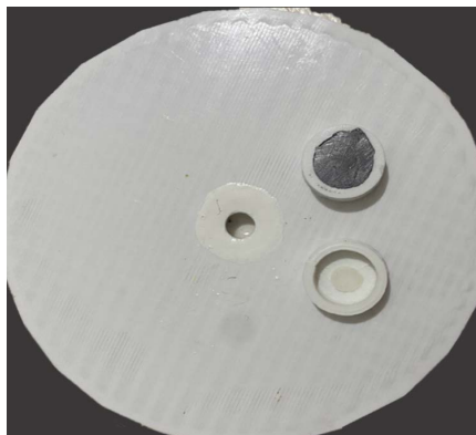
Figure 1. The platform was painted with white nail polish around the well so that the researcher could place the cap in the same place for every trial. This made measuring distance more accurate and kept the apparatus the same for every trial. The caps in this picture are both flipped upside down. The heavy cap was filled with lead and the light cap was empty. When turned right side up, the two caps were indistinguishable from each other.
