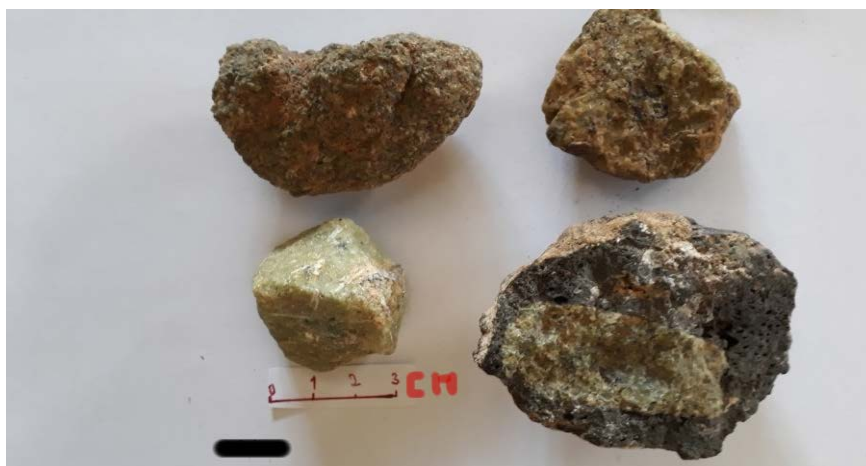
Figure 3. Different forms of xenoliths of olivine as granular or equidimensional or embedded within the scoriaceous materials.
