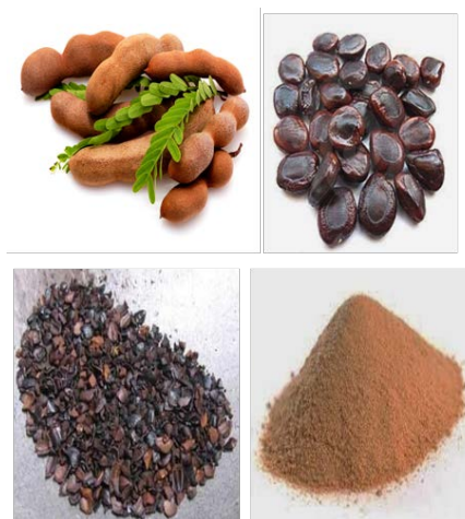
Figure 2. Separation of tamarind seed coat for extraction of tannin.
