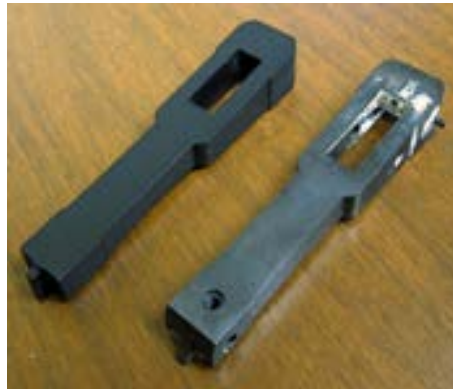
Figure 7. Part on left shows impregnated coated part and part on right shows breakdown of coating without impregnation [4].
