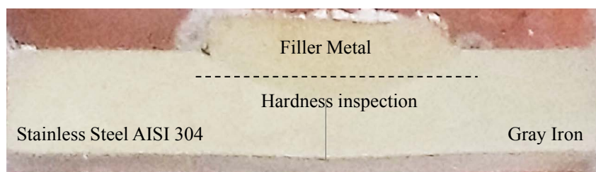
Figure 1. Cross section of one welded sample in polished condition.
