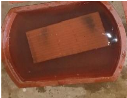
Figure 20. Submerged brick during an absorption test in a pan.
