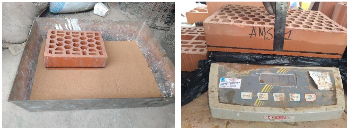
Figure 21. Brick subjected to the capillarity absorption test.
