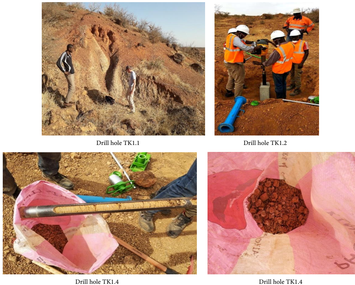
Figure 3. Illustrations of some of the manual drilling carried out.
