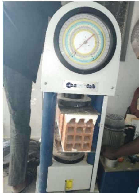
Figure 23. Press used for the determination of compressive strength.
