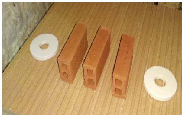
Figure 17. Samples of bricks after firing at 950°C.
