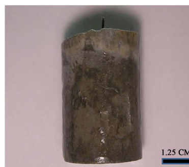
Figure 6. Day-4. Specimen subjected to a low ranging electric field. 24-nm, positively charged, alumina-coated, silica sol treatment, was applied with a starting electric field of 0.4 V/cm. See Table 3 . Submerged portions of the specimen were not covered with coagulated particles.
