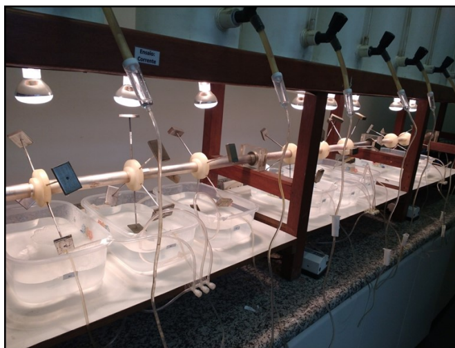
Figure 1. Experimental arrangement of the CEBELCOR test.
