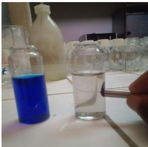
Figure 1. Separation of biochar/Fe 3 O 4 from the rest of the liquid solution by a magnet.
