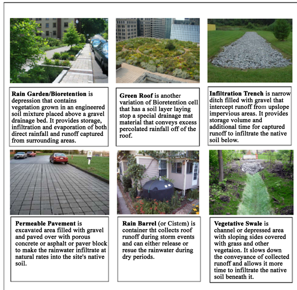
Figure 5. Description of typical LID measures in urban storm water management systems [61].
