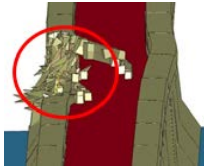
Figure 9. Maximum dynamic deformation of the guardrail.
