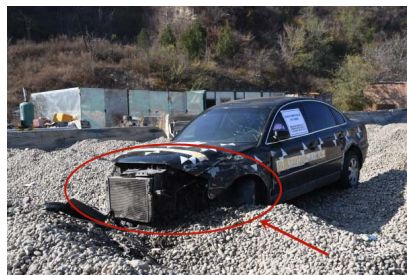
Figure 21. The situation after the barrier collision.
