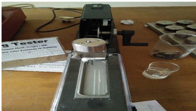
Figure 3. Testing procedure of color fastness to rubbing.
