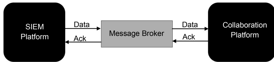
Figure 2. High-level architecture for Alert Distribution.
