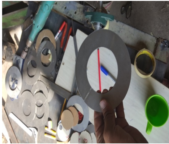
Figure 1. The helix before welded on shaft.
