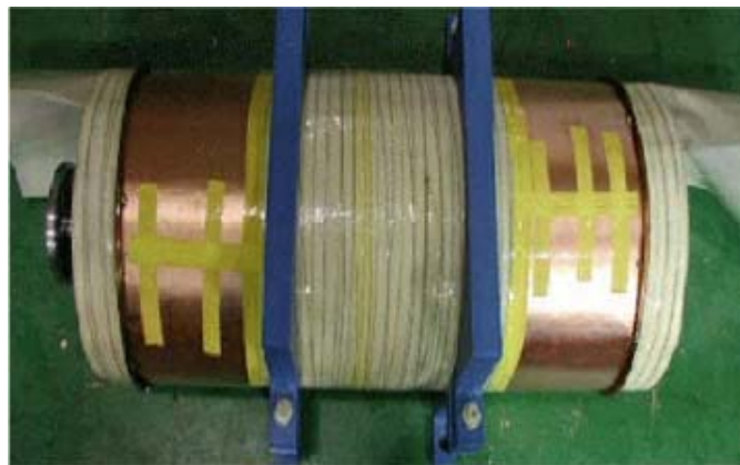
Figure 2. Air core pulse transformer.
