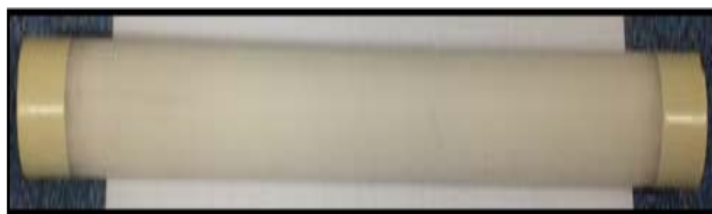
Figure 2. An unmodified commercial alumina membrane support.
