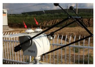
Figure 3. Solar tracker and direct radiometer.
