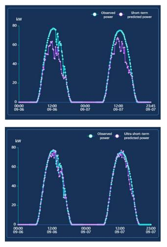
Figure 4. Observed and predicted power of short-term and ultra-short-term measurement results.
