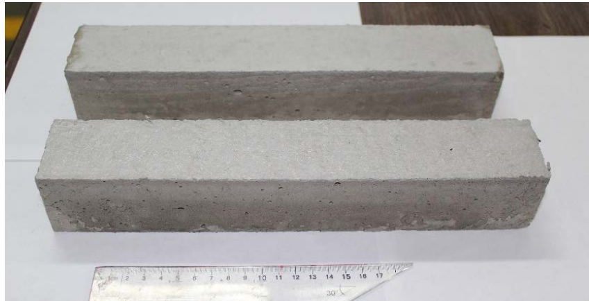
Figure 1. Continuous concrete bars of 5 cm (height) × 5 cm (width) × 30 cm (length) obtained after 24 h from casting.
