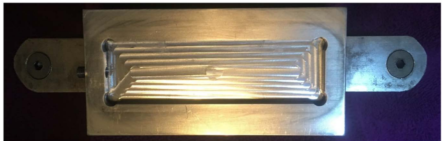
Figure 6. This is a bottom view of the holder showing where the specimen is held. The depth of the slot where the specimen is placed was slightly less than the specimen thickness.
