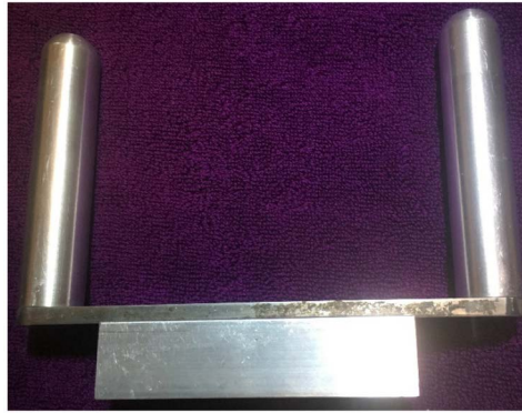
Figure 5. A picture of the specimen holder created to hold the specimens in place during grinding and polishing. There are two spread-out handles for the holder to assist in applying even pressure during grinding and polishing (to attain flat surfaces).
