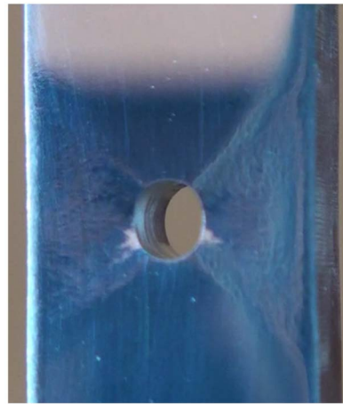
Figure 12. Angled picture of one-hole sample showing shear bands forming in a X pattern.
