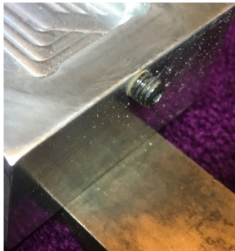
Figure 7. Shown here is a set screw on one end of the holder that is used to prevent any movement of the specimens during grinding and polishing.
