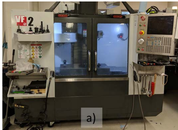
Figure 1. The CNC machine used in cutting the dog-bone specimens used in the tensile experiments.
