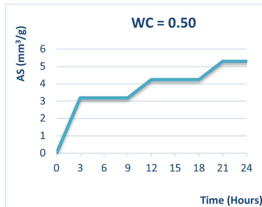
Figure 14. Evolution of autogenous shrinkage with time at w/c = 0.50 .
