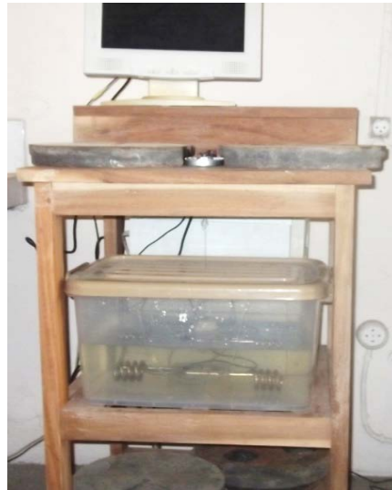
Figure 3. Set-up for the measurement of volumetric deformations.
