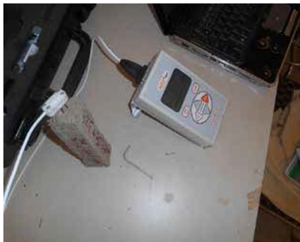
Figure 5. Thermal characterization in process with Decagon Devices KD2 Pro Thermal Properties Analyzer.
