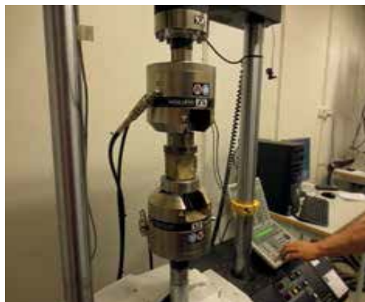
Figure 6. Compression testing on a cubic-shaped sample with an Instron 8516 machine.
