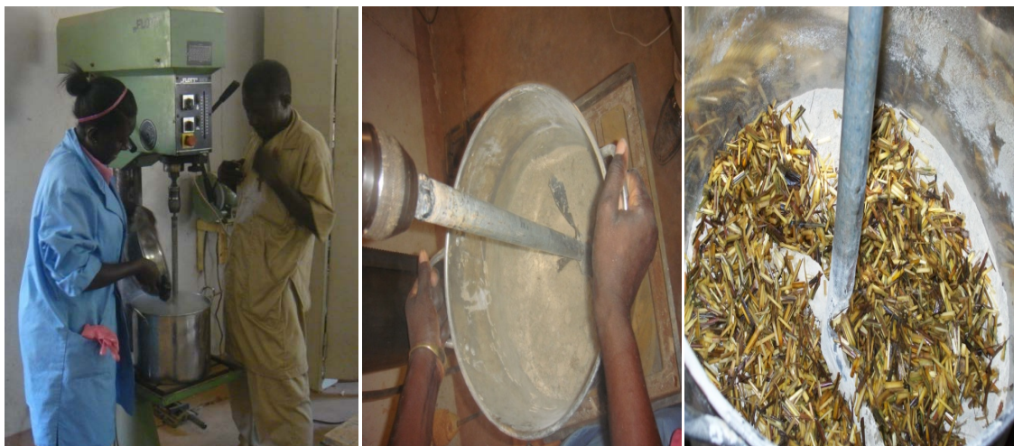
Figure 1. Mixing by shearing with a FLOTT M3 ST drilling machine which has been provided with a finned rod.
