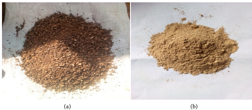
Figure 1. (a) Crushed coconut shell powder and (b) Coconut shell ash.
