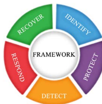
Figure 7. It shows the NIST cyber security framework which consists of five concurrent and continuous functions—identify, protect, detect, respond, recover (NIST, 2018).
