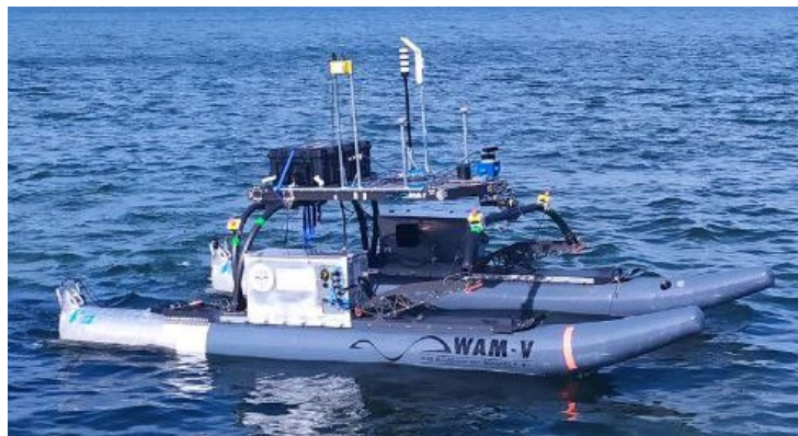
Figure 1. WAM-V unmanned vessel equipped with Velodyne VLP-16 sensor.
