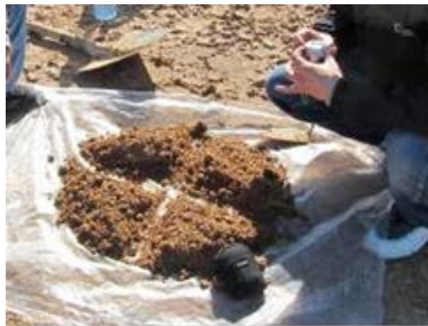
Figure 4. Mixing of the samples from the 4 corners to represent one soil sample.
