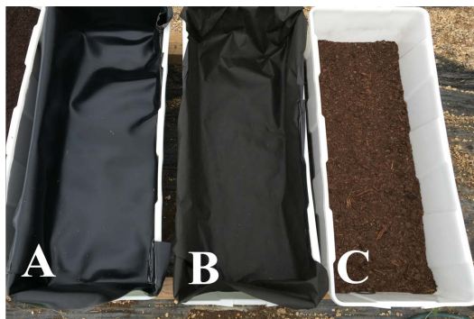
Figure 4. Simulated raised bed barriers applied to containers. Contaminated media sealed by selected barriers up to the top of each container's edge ((A) neoprene rubber; (B) landscape fabric; (C) no-barrier control).
