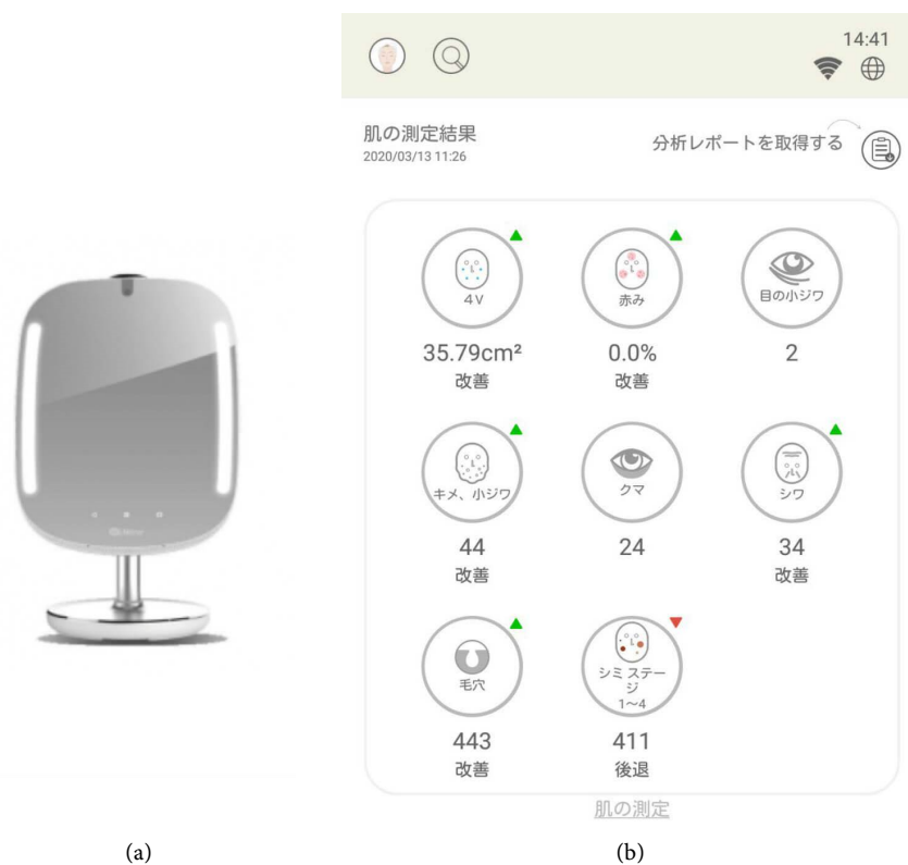
Figure 3. HiMirror-Professional. (a) HiMirror-Professional. HiMirror Professional uses the photos of patients, analyzes the skin, and saves the data. It can acquire daily skin data, and care for especially necessary sites; (b) Diagnosis. Seven items are measured; stains, pores, wrinkles, fine lines, roughness, redness, and dark circles.
