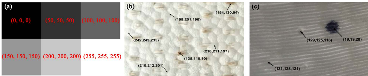
Figure 3. The three-component gray value of each area. (a) Schematic diagram of the same three-component gray value; (b) Three-component gray value of scorch defect; (c) Three-component gray value of dirt defect.
